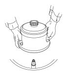
**NOTE** If the rotor sticks to the drive spindle, screw the short end of the rotor lifting handle assembly into the threaded opening to force the rotor off of the drive spindle hub. Lubrication of the centrifuge drive spindle hub with Spinkote should prevent the rotor from sticking on all centrifuges except Avanti J series. Avanti J series centrifuges have acetal rings on the spindle hubs to prevent sticking and do not require lubrication.
