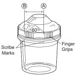
To tighten, turn the lid from (A) to (B). Tightening down the lid more than this will make it difficult to remove.
