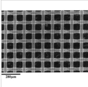
**10.0 µm pore size, hydrophilic nylon membrane,
