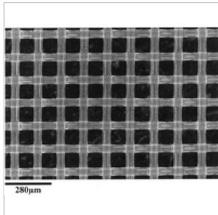
**20.0 µm pore size, hydrophilic nylon membrane,
