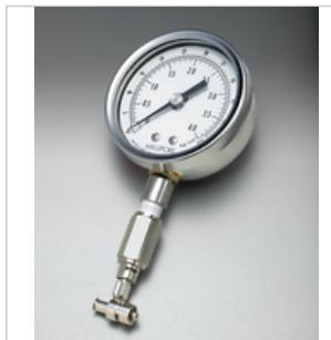
For bubble-point testing of small filter units.
