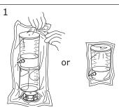
Open the Stericup® or Steritop® bag at the notched edge. The Stericup® filter funnel is packaged fully tightened onto the bottle and requires no further tightening.
