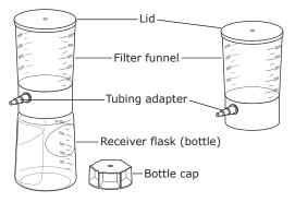
Stericup® and Steritop® systems come in different sizes to handle different sample capacities; the system components are the same except for capacity.
