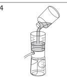
Remove lid (if not already removed) and pour sample into funnel. Replace lid, if desired, and apply vacuum until filtration is complete.
