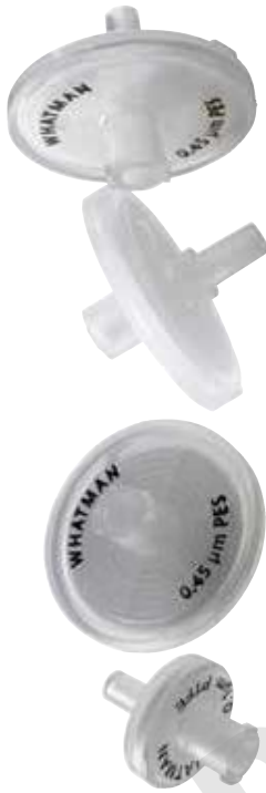
Fig 11. Puradisc filters are produced from pigment-free polypropylene with standard inlet (female luer lock) and outlet (male luer) connections (unless otherwise stated).
