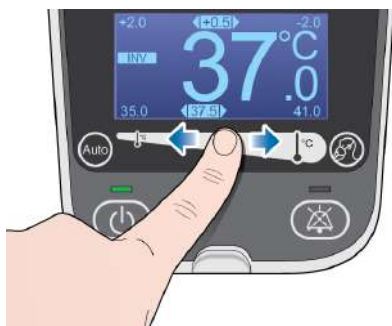
Figure 11. Adjusting Chamber exit temperature
