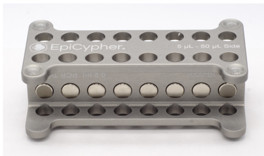
FIGURE 1 Magnetic Separation Rack, front view. Note that the 5 - 50 \mu L is up, and that the magnets are toward the bottom of the rack, so that the beads will be sorted near the bottom of the tubes.
