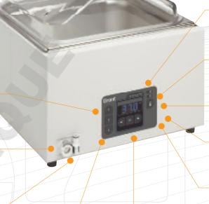
Three programmable temperature presets – allows commonly used temperatures to be quickly selected User calibration – single or dual-point for optimum accuracy at your working temperatures Clear, wide-angle viewing LED display - instant reassurance of bath status
