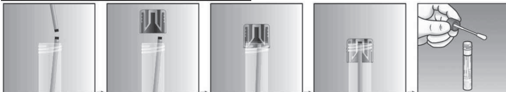
Fig 3. Capture of broken swab applicator stick by FecalSwab™ tube cap
