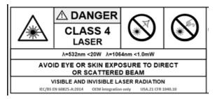
Figure 2 Illumina field service engineer laser warning label
