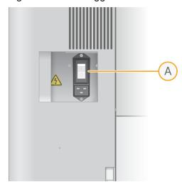
2. Press the power button on the right side of the instrument.
