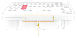
2. To detach the position #3 and #8 wells from the reagent cartridge, press the tab, and then push the well upward.
