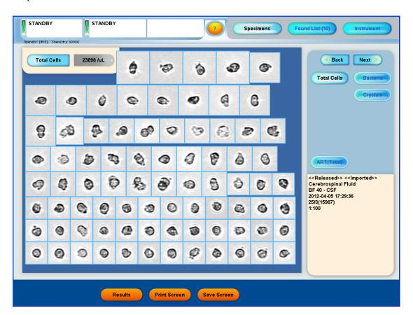
In the above screen, the operator is able to reclassify images that do not belong in that category. For example, in the Total Cells screen, the operator can move images to the Bacteria or Crystals categories to indicate that these particles may be present and tag the sample for confirmatory testing, or the operator can select **ART (Total)** to reclassify images as artifacts.
