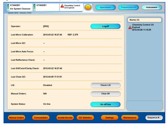
Figure 17.2 Red Alarm for Use of Expired Quality Control Material - Example
