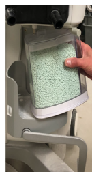
Figure 1. Presenting SmartCan to lifter dish
