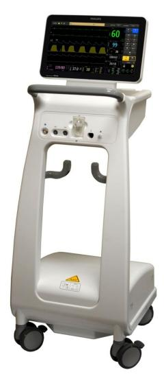
The Expression Model MR400 MRI Patient Monitoring System is designed to assist clinicians in monitoring patient vital signs in the dynamic magnetic resonance environment. The Expression Model MR400 MRI Patient Monitoring System combines wireless communication, radio frequency shielding and digital signal processing to address the challenges associated with patient monitoring in the MR environment.
